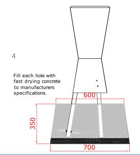
Foundations should not present a hazard. These foundations are recommended as a guide, for more information on foundation details for various surface see Part 1 of BS EN 1176.
