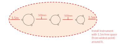
Diembes will arrive on site in pre set heights. In ground fixing depth 300mm for all 3 Drums.
